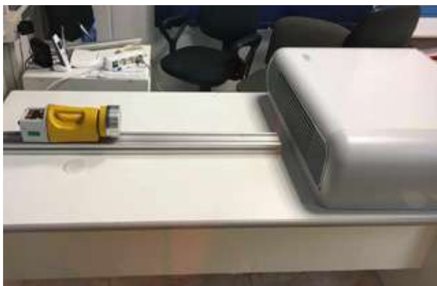
Figure 1 - harvesting of aerosol with the use of SAS Super 100
