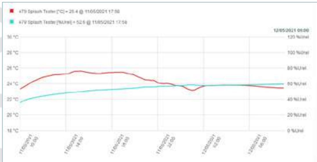
Temperature trend (red line) and humidity trend (blue line) inside the case
